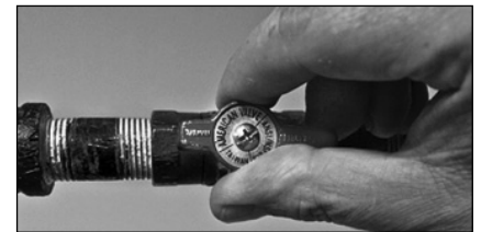
Figure 45 - Gas valve in "on" position.
