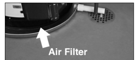
Figure 41 - Clean air filter periodically.
