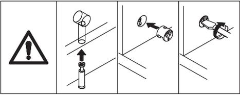
Attach board 11 to board 13, add cam lock(B) into and turn clockwise to tighten as shown.
