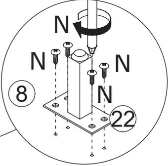
Fix leg 23 to board 8 with screw(N) as shown.
