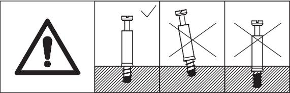
Screw eccentric rod(A) into board 15.
