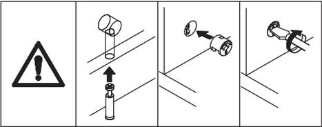
Attach board 11 to board 15, add cam lock(B) into and turn clockwise to tighten as shown.
