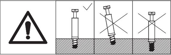
Screw eccentric rod(A) into board 13.
