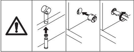
Connect board 11 to board 12 and 14, add cam lock(B) into and turn clockwise to tighten, and fix board 13 and 15 to the cabinet with screw(D) as shown.
