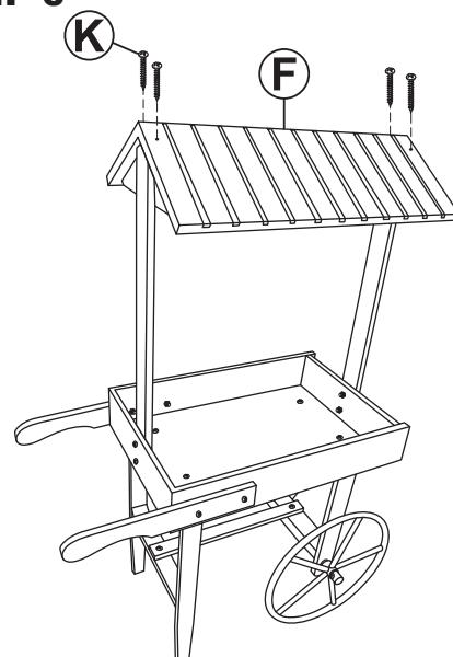
Place Roof (F) on the support posts and secure using four Screws (K).
