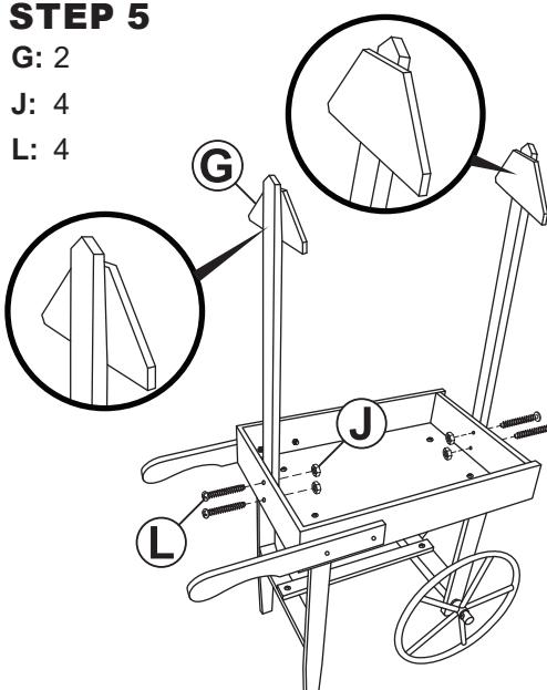
On the handle side, install one Support Post (G) on the inside of the planter box using two Bolts (L) and two Nuts (J).
