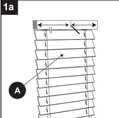
2. Slide mounting brackets (AA) onto each end of the blind (A) headrail. Position blind (A) in sidelight and align center marks. Mark position of mounting brackets (AA) with a pencil.
