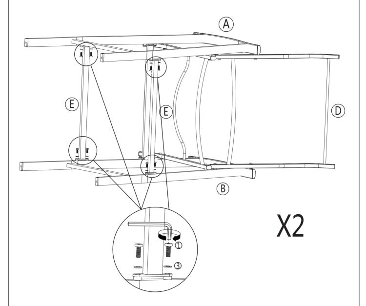
Fix part E to part A and part B with eight M6x15mm Screws (1) and Flat Washers (3).Use (6) Allen key. **DO NOT YET TIGHTEN.**
