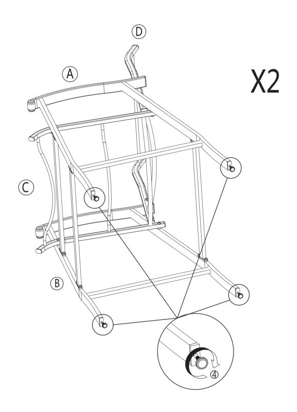
Rotate part (4) into bottom of part A and part B,do this four times.
