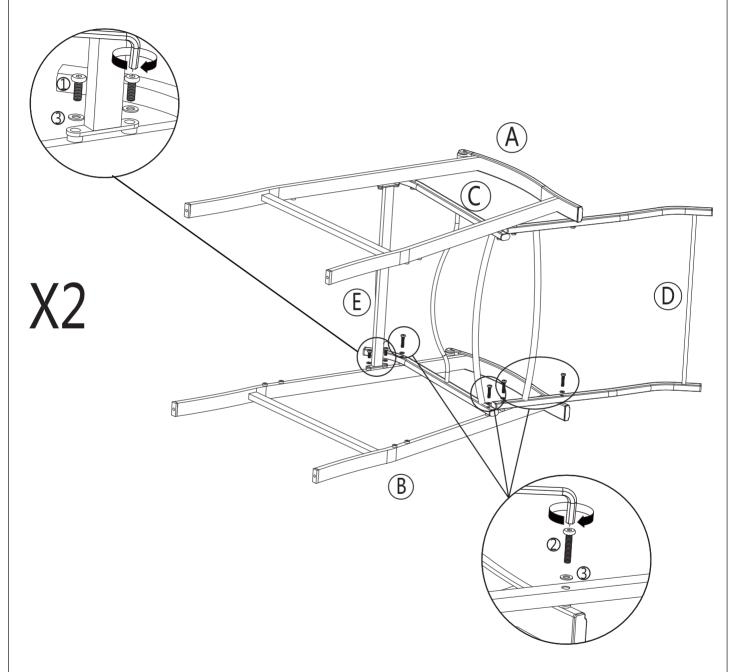
Fix part C and part D to part B with four M6x30mm Screws (2) and Flat Washers (3).Use (6) Allen key. **DO NOT YET TIGHTEN.**
