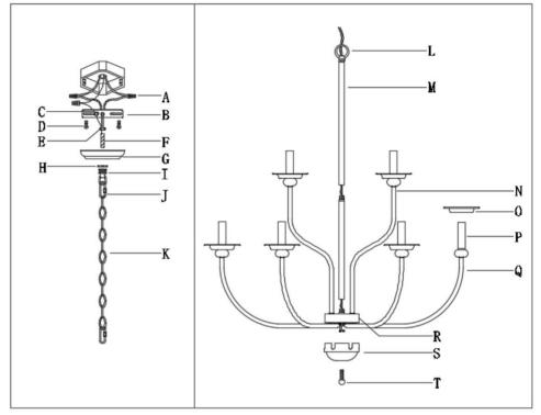
Step A1:Carefully thread stem(M) onto the top of wire house (R) until snug.
