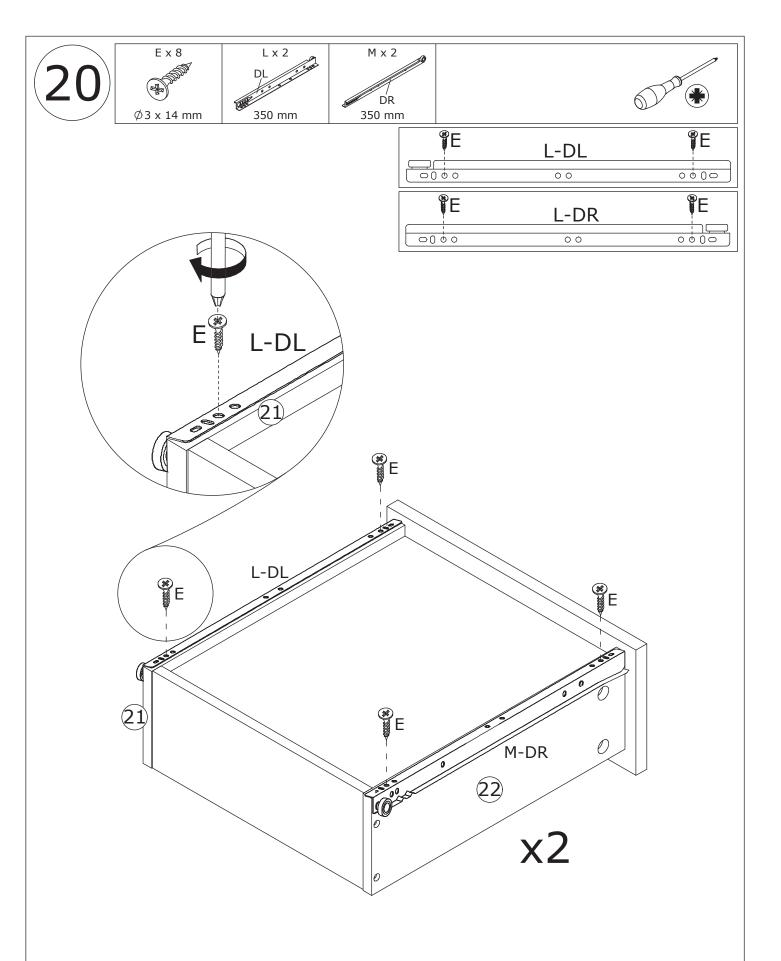
Fix track(DL) and (DR) to board 21 and 22 with screw(E) as shown.
