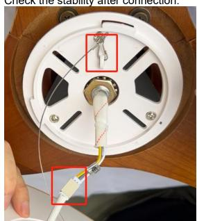
5. Spin the light box to the Motor and lock it. Double check the Sturdiness.
