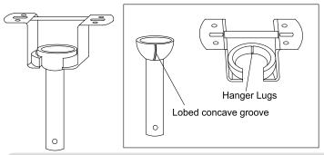
Lift the fan assembly onto the mounting bracket. Ensure the registration slot of the hanger ball is positioned on the stopper of the mounting bracket to prevent the fan from rotating when in operation.
