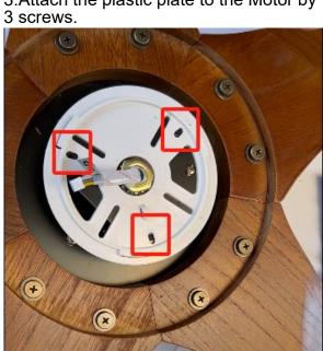
2.Rotate the white plastic plate, you will find the safety rope and LED wire in the light plate.
