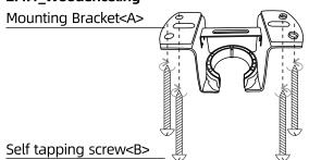
For wooden ceiling, use wood screw to drill on the wooden beam or the "junction box" to fix the hanging bracket (selection is made according to actual requirements of the customers).
