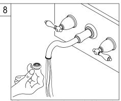
8. Remove aerator and turn on both hot and cold valve, let water run for at least 1 minute, this will clear any debris remaining on the waterways, replace aerator.
