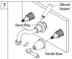
7. Thread handle bases and attach handles. Make sure handle operates freely without any resistance and in the desired direction, adjust as necessary, Apply a bead of silicon based caulking to the perimeter of the spout ring and slide back to the wall, clean any excess caulking.
