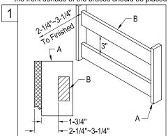
1. Prepare location by securing 2 horizontal wood braces allowing for a 3" clearance in between the braces, the front surface of the braces should be placed at 2-1/4"~3-1/4" from the finished wall surface.
