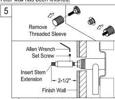
5. Remove both threaded sleeves, insert stem extension and make sure that the tip of the stem extension is approximately 2-1/2" from the finished wall surface, secure by tightening the set screw.
