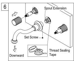
6. Attach spout extension if needed for wall thickness more than 1" and insert both extended threaded sleeves, apply Teflon tape to the spout extension and thread spout, make sure to thread the spout fully and then back thread until the spout is facing downward, secure with set screw at the back of the spout.
