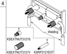
4. Weld both hot and cold water supply lines onto valve inlets. If your wall has a thickness of more than 1" you will need to replace the short stem extension and short threaded sleeve with KSRP3121EXT (long stem extension), KSEXTNUT3121V (long threaded sleeve) and KSEXTNUT3121S (spout extension) to accommodate the wall thickness.
