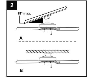
3. Check to make sure blades (G) will be at least 30 inches from any obstruction. Check downrod (A) length to ensure blades (G) will be at least 7 ft. above the floor.
