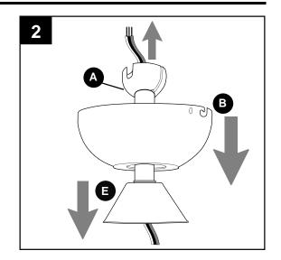
Slip downrod (A) into motor housing yoke, align holes and re-install pin (M) and clip (N). Tighten set screws in motor housing yoke and then tighten preassembled nuts on the set screws.
