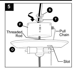
Connect WHITE wire from light kit fitter (O) to WHITE wire from switch housing (F). Connect BLACK wire from light kit fitter (O) to BLUE (or BLACK) wire from switch housing (F). Make sure that molex connections snap together securely.
