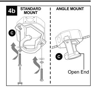
Remove preassembled motor screws/lock washers (J) from underside of motor housing (D). If there are plastic motor blocks installed with the motor screws/lock washers (J), discard the plastic motor blocks.
