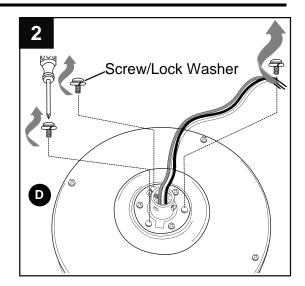
3. Pull wires up through hole in the middle of the canopy (B) and attach canopy (B) to motor housing (D) using the three previously removed screws/lock washers.
