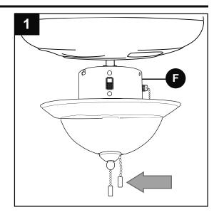
2. If applicable, the pull chain located in the middle is used to turn the light ON or OFF.
