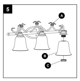
Install light bulbs (not included). Use three 100-watt max. standard-base incandescent bulbs or halogen/CFL/LED equivalents.
