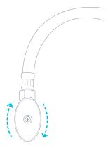
3. Connect the Metal Adapter with Valve between the cold water supply line and cold water valve.
