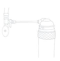
5. Remove the end of the PE Tubing from the Filter Flushing Adapter by pressing in on the push connect ring and pulling out the PE Tubing.
