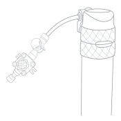
5. Using the Small PE Tubing, connect the right side inlet of the first Filter Adapter to the left side inlet of the second Filter Adapter.
