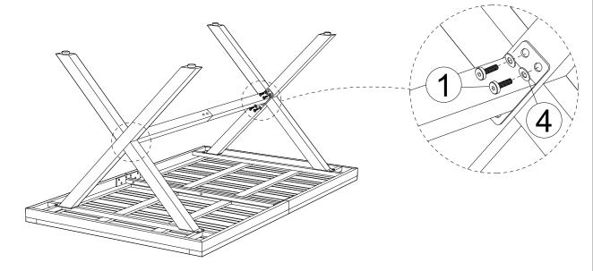
Connect The part from Step 3 & The part from Step 4, tighten Bolt (1) & Flat Washer (4) with Allen Key (9).
