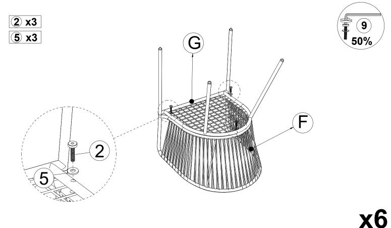
Connect the Seat Chair Frame (G) & The Back Chair Frame (F), tighten Bolt (2) & Flat Plastic Washer (5) & Allen Key (9).
