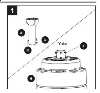
2. Insert the downrod (A) through the canopy (E) and yoke cover (F). Feed the wires from the fan through the downrod (A). Depending on the length of downrod you use, you may need to use the 36-inch lead wire (K) to accommodate a 36 or 48-inch downrod (sold separately). When necessary, connect the 3-pin extending from the center of the downrod to one end of the 36-inch lead wires. **Note:** The downrod included with this fan will not utilize the 36-inch lead wire (K).
