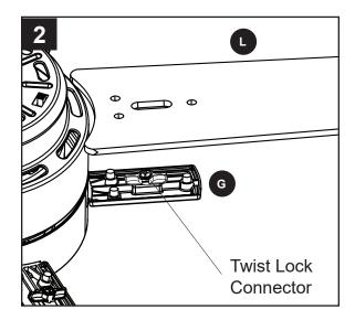
3. Rotate the twist lock connector so that it is perpendicular to the hole in the blade (L). Repeat for the remaining blades (L) and blade arms (G).
