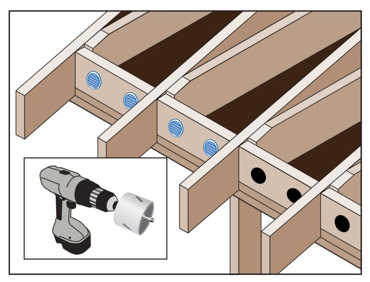
Mini Louvers are used to seal existing rafter/bird block vent holes to maximize airflow while protecting against rodent and insect invasion.
