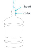
7. If you are using a 3 gallon bottle rather than a 5 gallon bottle you can adjust probe by pressing the two tabs at the head of the probe and sliding the collar down to the neck of the bottle.
