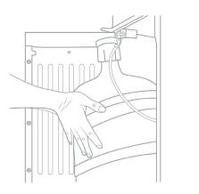
8. Push the head down until the tube hits bottom of the bottle.
