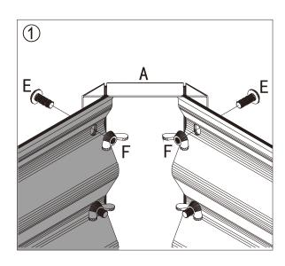
$\ \textcircled{1}$  Attach 2 Corner Connectors #A to 1 Short Sheets #B with 8 screws #E, and secure with 8 wingnuts #F .
