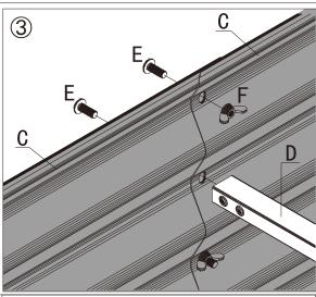
③ Overlap the 2 halves of the garden bed, then connect with 6 screws #E, and secure with 6 wingnuts #F. Leave the second set of connector holes empty.
