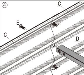
④ Attach the Bracing Rod #D with 2 screws #E.
