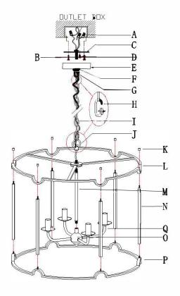
Step A1: Connect the upper iron frame (L) and lower iron frame (P) together with a tube (N) and secure with screws (K).
