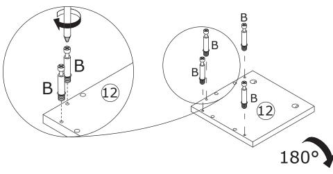
Screw eccentric rod(B) into board 12 at first.
