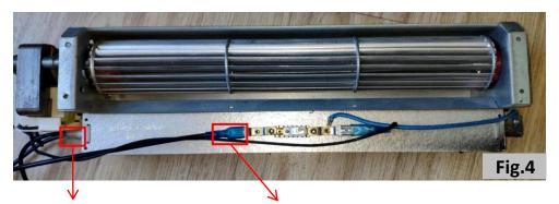
Here are two sets of heating. If one wire disconnects, one set will does not heat.
