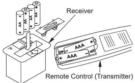
**Figure 21 - Installing Batteries in Remote Control and Receiver**
