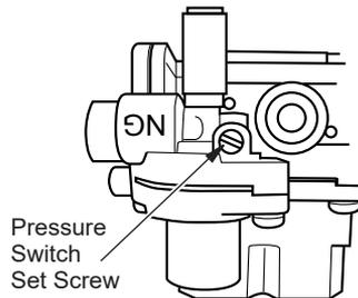
**Figure 34 - Gas Regulator Pressure Switch**
