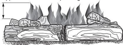
**Figure 30 - Correct Burner Flame Pattern**
