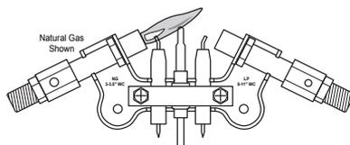
**Figure 28 - Correct Pilot Flame Pattern (Natural Gas shown)**
