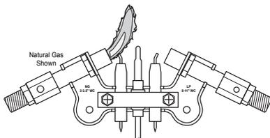
**Figure 29 - Incorrect Pilot Flame Pattern (Natural Gas shown)**
