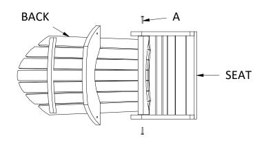
1) Insert (1) "A" Bolt into Lower Hole on Each Side to Attach Seat to Back. Make Sure the Back is Fully Upright. Make Bolts Snug, but Do Not Overtighten.
