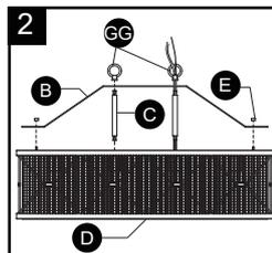
3. - Determine length of chains(FF) needed to achieve desired fixture height. (To remove excess chain section, use pliers to bend link open.)
