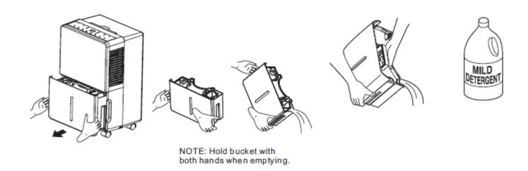
NOTE: When the bucket is full or removed from the machine, the compressor will turn off, but the fan will continue to run for a few minutes. This is completely normal. The dehumidifier will not be removing moisture from the air at this time.
