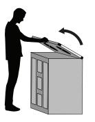
Lower the countertop so that it lays flat on the cabinet, while supporting it from theside and front. Be careful not to catch your fingers under the countertop. It is best to lower the countertop by supporting from the front as it comes down onto the cabinet.
