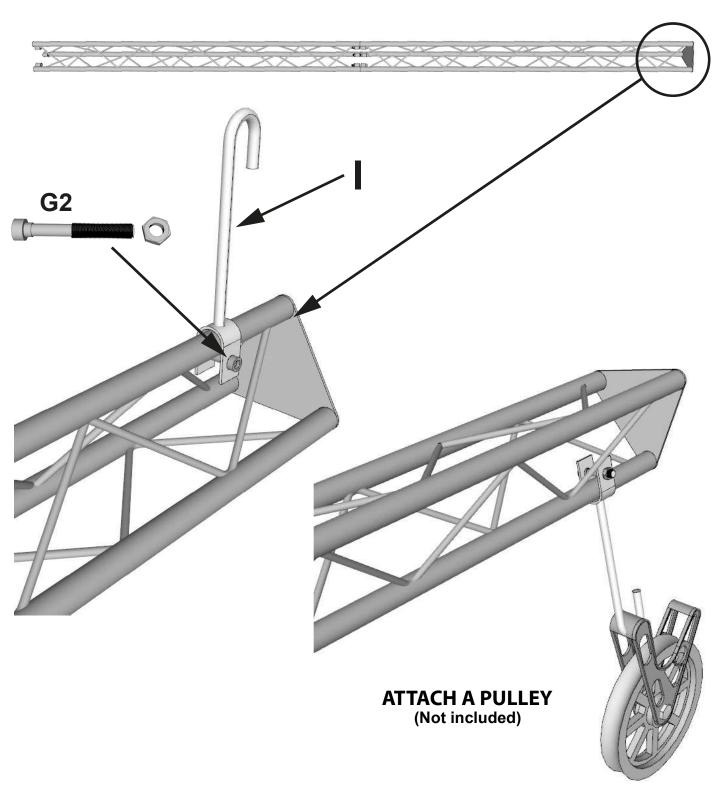
STEP 6 - INSTALLING SECTIONS "C" AND "D" ON SECTION "B"
