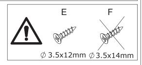
Assemble door 24 to board 4 and 5 by fixing hinge with screw(E) as shown.
