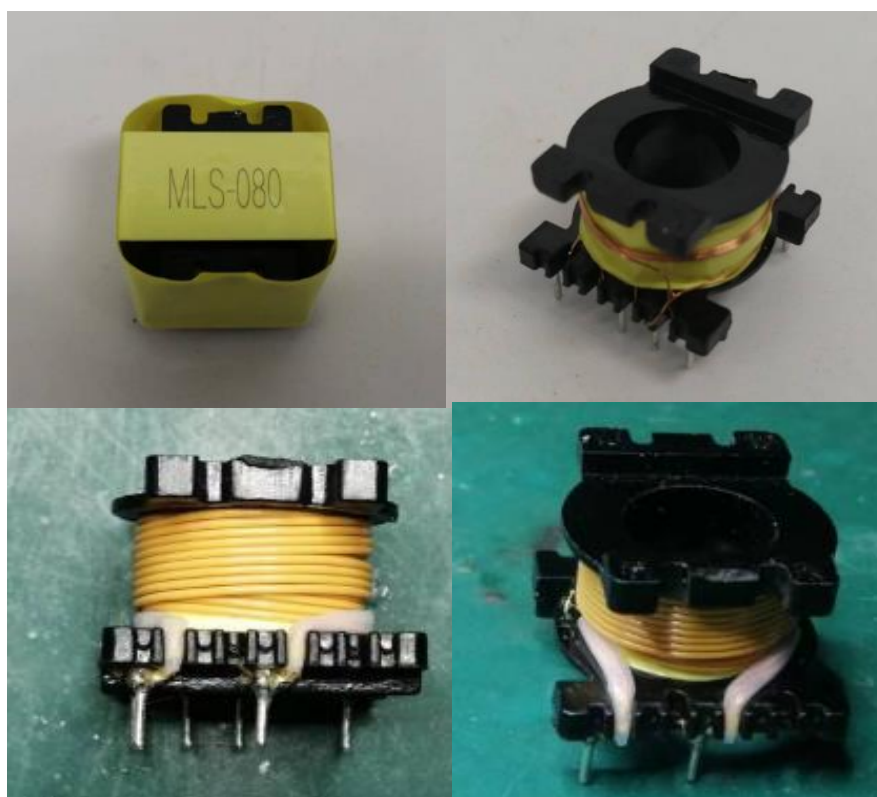
Photo 73 - Internal view of Transformer (T1) model MLS-080
