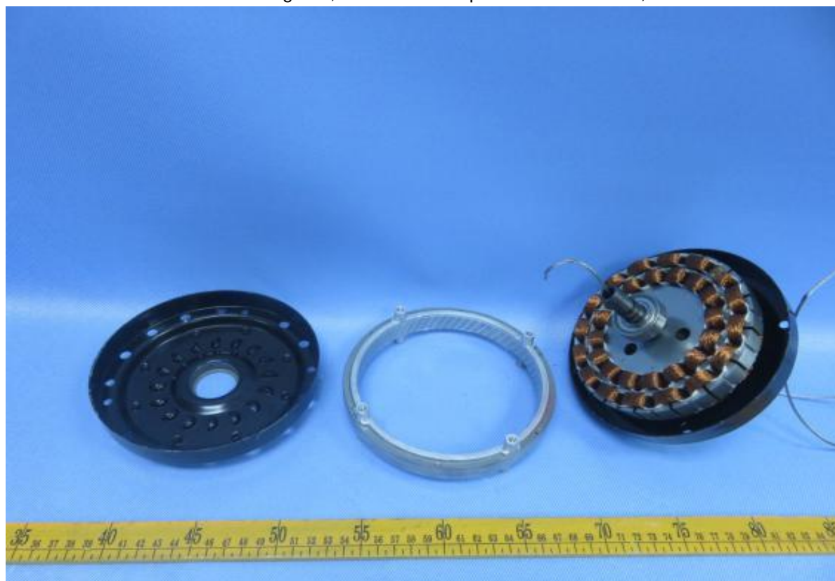
Photo 32 - Internal view of Ceiling Fan, all models except models KBS-6005, KBS-5219.
