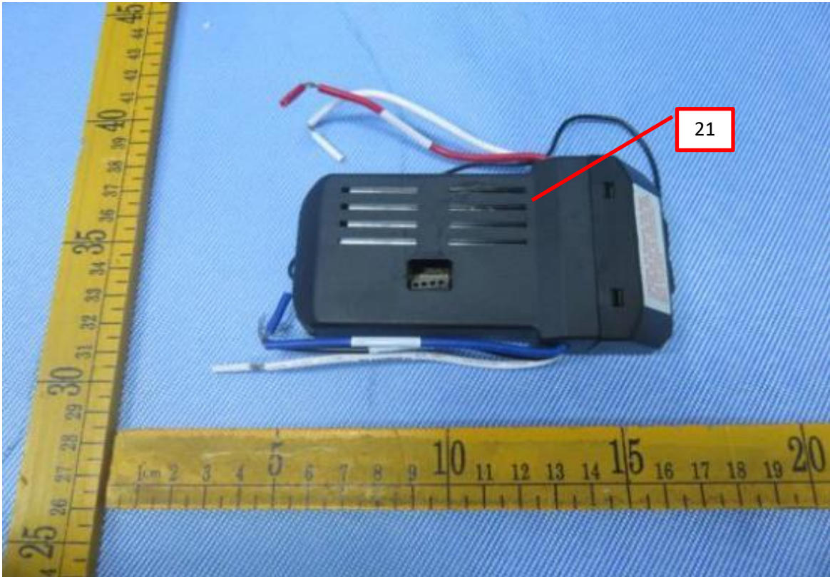
Photo 33 - Speed control of Ceiling Fan for models KBS-Y4203, KBS-Y4296, KBS-Y4294, KBS-Y4274, KBS-Y4297, KBS-Y4299, KBS-Y4240, KBS-Y4298, KBS-Y4295, KBS-Y4216, KBS-5226
