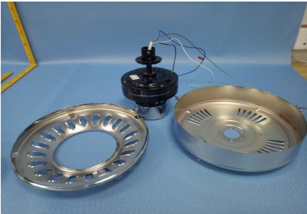
Photo 38 - Internal view of Ceiling Fan, model KBS-5270
