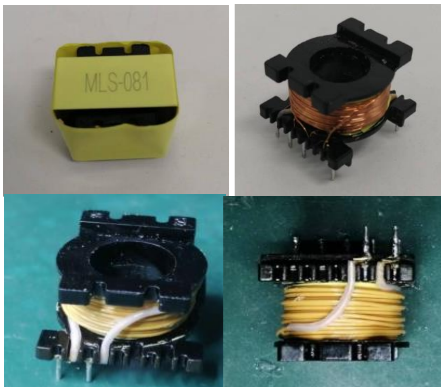
Photo 74 - Internal view of Transformer (T2) model MLS-081
