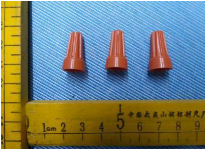
Photo 35 - Field wiring terminals of Ceiling Fan
