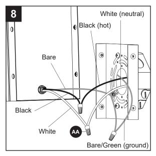
Wrap electrical tape (not included) around each individual wire connector (AA) down to the wire. Turn the spliced/taped wires upward and gently push the wires and wire connectors (AA) into the outlet box.
