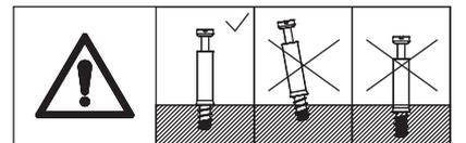
Screw eccentric rod A into board 13.
