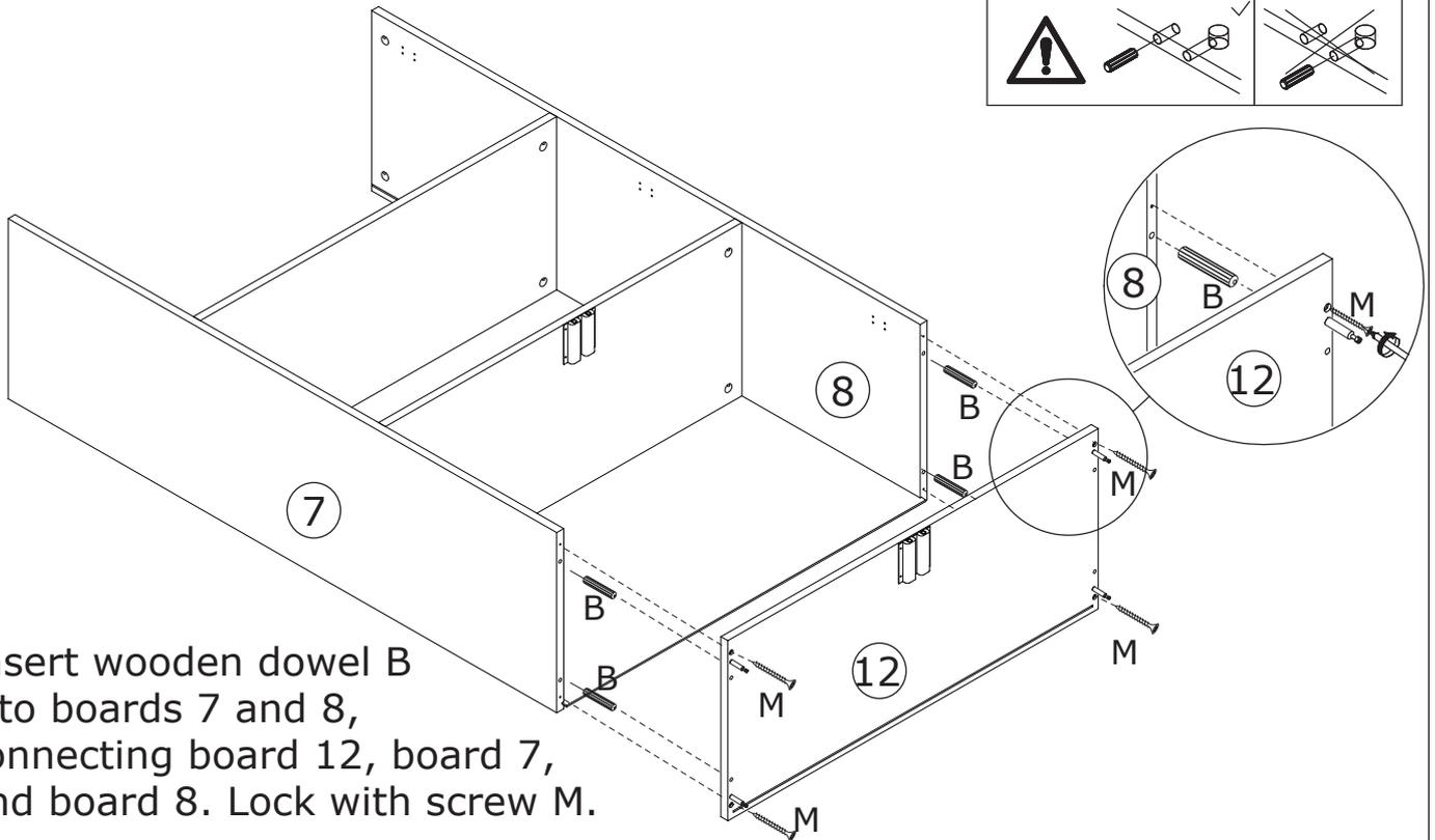
Insert wooden dowel B into boards 7 and 8, connecting board 12, board 7, and board 8. Lock with screw M.
