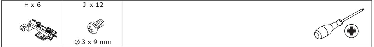
Fix hinge H onto door 14 with screw J.
