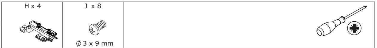
Fix hinge H onto board 15 with screw J.
