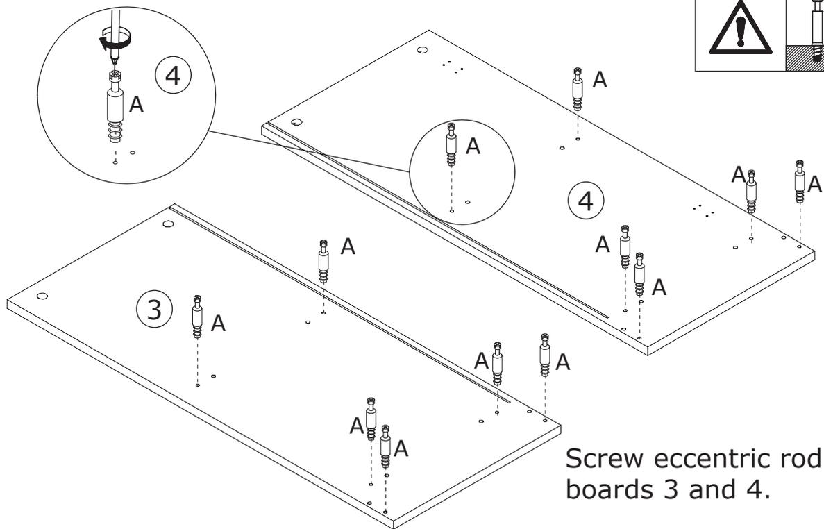
Screw eccentric rod A into boards 3 and 4.
