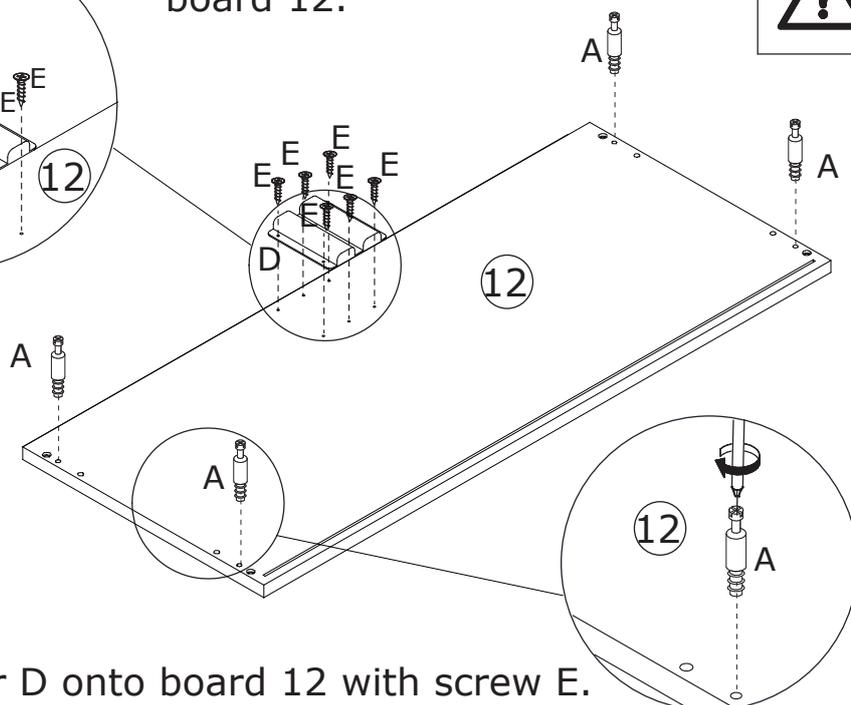
Fix rebounder D onto board 12 with screw E.
