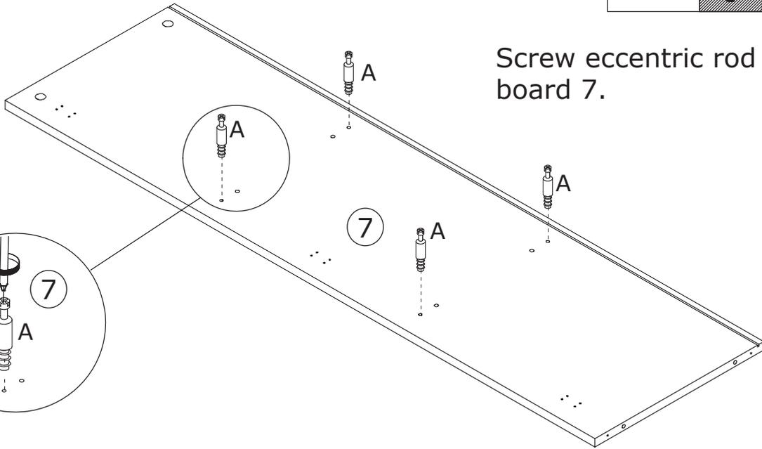
Screw eccentric rod A into board 7.
