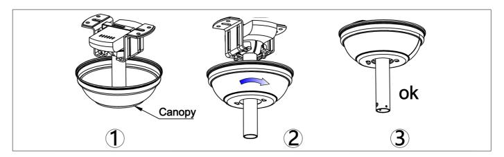
Raise canopy to hanging bracket, aligning loosened screws in hanging bracket with slotted holes in canopy. Twist canopy to lock. Re-insert screws and secured all screws with screwdriver.
