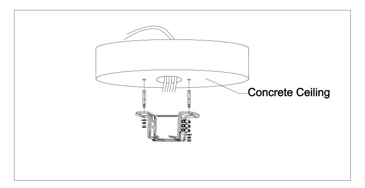
Please drill  $\phi 8mm$  hole on the concrete ceiling, and insert the bolt. Align bracket with the hole, then tighten with nut.
