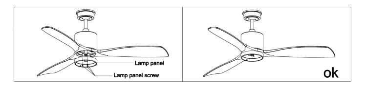
Unscrew a set screw. Attach the LED pan up to the bottom of the fan by inserting the other two set screw heads into key hole slots, rotate it to place, then secure the previous set screw by aligning screw hole and the hole at the bottom of the fan, tighten the rest two set screw to secure LED pan.
