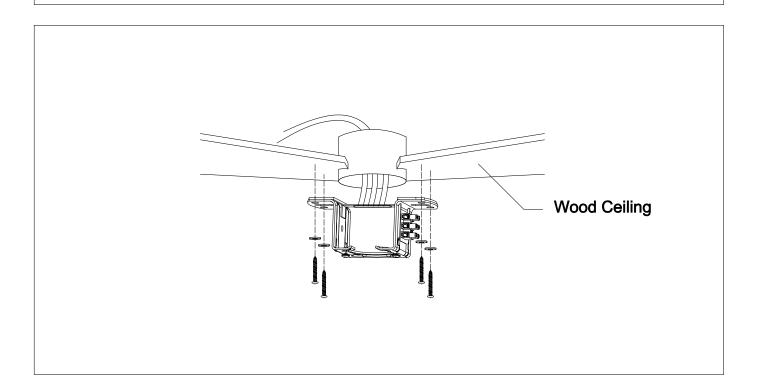
Please tighten the bracket in the wood ceiling with tapping screws.
