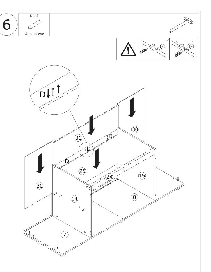
Connect board 31 to board 25 using wooden dowel(D) at first. Insert back board 30, 31 and 25 along available grooves as shown.
