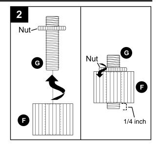
3. Insert adapter (F) into bottle so the 1/4 in. part of the threaded rod (G) faces down. Slide ring (E) and saddle (sold separately) over threaded rod (G), ensuring the open part of the ring (E) is turned down toward the bottle opening.
