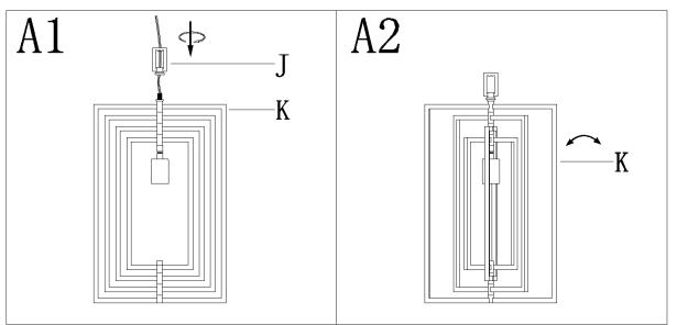
Step A1: Carefully thread the wire through the loop (J), and then screw the loop (J) to the top of the iron frame (K). Step A2: Adjust the iron frame (K) to the proper position.
