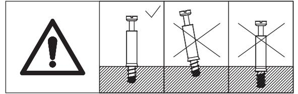
Screw quickfit screw(A) into corresponding holes in plate 9 as shown.
