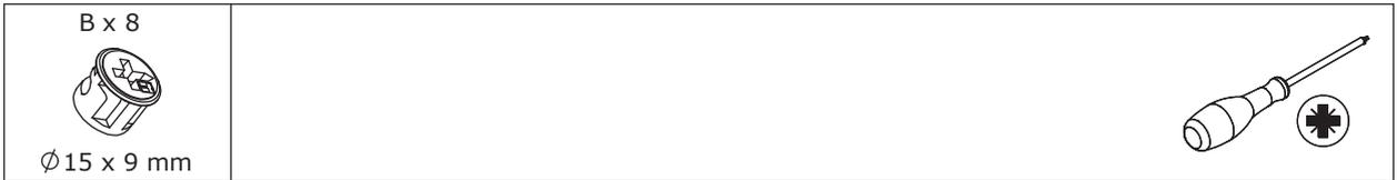
Attach drawer face plate 15 to the component, put cam lock(B) into holes in plate 20,21 and turn clockwise to tighten as shown.
