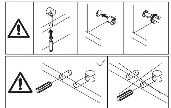
Connect plate 9 with plate 10 using wooden dowel(L), put cam lock(B) into holes in plate 10 and turn clockwise to tighten as shown.
