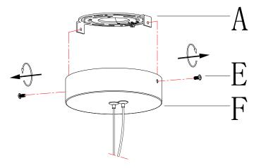
4 » Attach mounting plate (A) to the outlet box with mounting screws (D).
