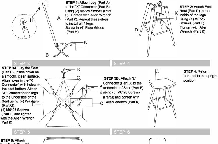
Seat Back (Part E) to the "L" Connector using (3) M6\*20 Screws (Part J) and tighten using the Allen Wrench (Part K)
