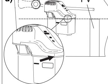
Verify corner of white cover and top of flush valve (FV) line up.
