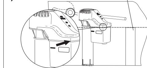
Press valve down until corner of white cover &amp; top of flush valve (FV) line up. Note: If tower style flush valve (TS), match fill valve water line to water line marked in tank (stain line).
