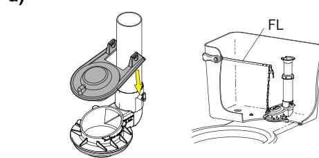
Remove old flapper. Install new flapper. Attach chain to flush lever (FL) with minimal slack.
