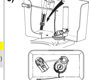
Place locked valve in tank so refill tube has direct path to flush valve.
