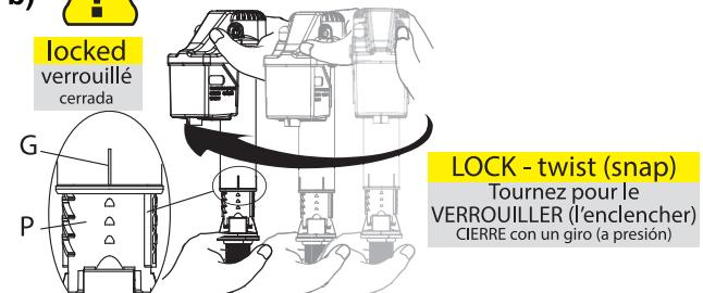
Twist upper half of valve clockwise to lock (snap). Groove (G) lines up with pegs (P). Keep locked.
