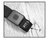
Slide the heart rate monitor onto your arm as shown. Make sure that the iFIT button (G) is facing upward. You must position the heart rate monitor under your clothes, against your skin, 2 to 3 inches (5 to 8 cm) above or below your elbow. Then, pull the free end
