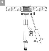
Position faucet on the installation surface. Fit flexible hoses through hole on countertop or sink.
