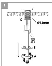
Ensure there is a Ø35mm through-hole on the kitchen counter. Remove the mounting nut (A) and washer (B) from the threaded shroud (C).
