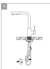
Connect pullout hose to quick connect and insert weight (loose-install).
