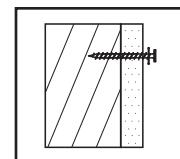
**DRY WALL:** Drill holes and secure to the wall with toggle bolts and a washer./**CLOISON SÈCHE**
