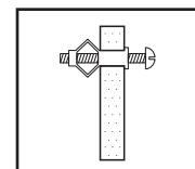
**CONCRETE WALL:** Drill 1/4 in. holes, insert #12 wall anchors and secure to wall with #12 x
