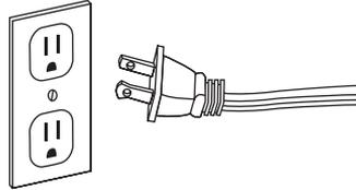
**⚠ WARNING:** It is normal for the power cord to feel warm to the touch. However, a loose fit between the outlet and the plug may cause overheating of the plug. If this occurs, try inserting the plug into a different outlet. Contact a qualified electrician to inspect the original outlet for damage.
