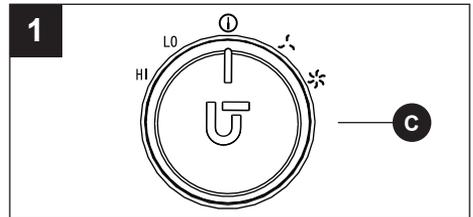
2. Select a heat or fan setting by turning the MODE dial on the control panel (C) to the "LO", "HI", "⓪", or "fan" position.
