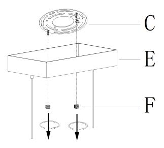
4 » Attach mounting plate (C) to the outlet box with mounting screws (B).
