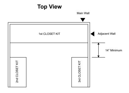
Closet kits can be installed in several layouts. Plan your layout before starting installation.
