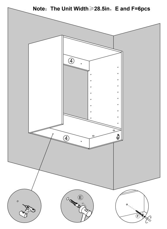
DETAIL HOLE FOR WALL FIXING Note: hammer is not included.
