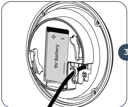
**Install the battery** into the lock face. You will hear 1 beep when the battery is correctly installed.
