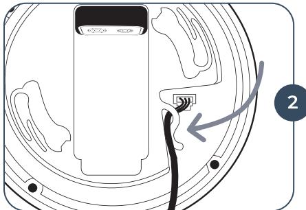
**Secure the wire** into the clip to prevent it from moving.
