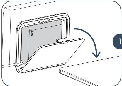
On the inside of the safe, **locate the battery compartment** in the top left corner.
