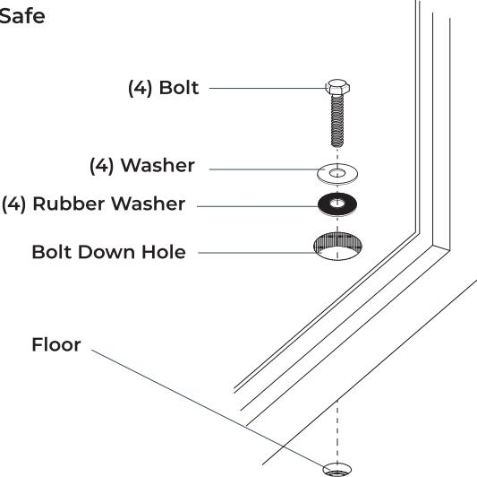
**WARNING:** Always ensure the safe is in an isolated and dry area. Never place the safe in direct contact with a wet floor. We recommend using a moisture/protective barrier to prevent damage.
