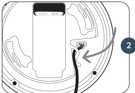
**Secure the wire** into the clip to prevent it from moving.
