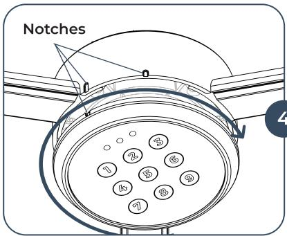
**Align the notches** on the left of the lock face back, push in, and rotate clockwise until you feel it click in place at the center notch.
