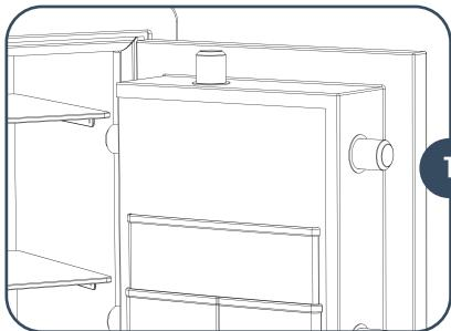
With the door open, **extend the bolts by turning handle counterclockwise**. This will ensure that the door stays open during programming process.
