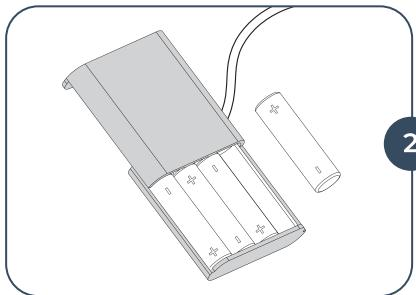
**Slide open the cover** on the battery pack and install the batteries. Replace into the battery compartment.
