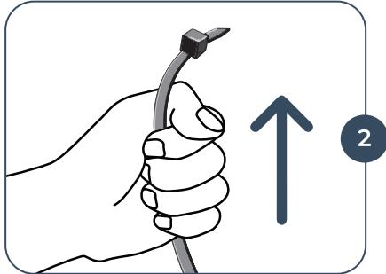
**Grab the larger end** of the zip tie (at the front) and **pull in an upwards motion** to remove it.
