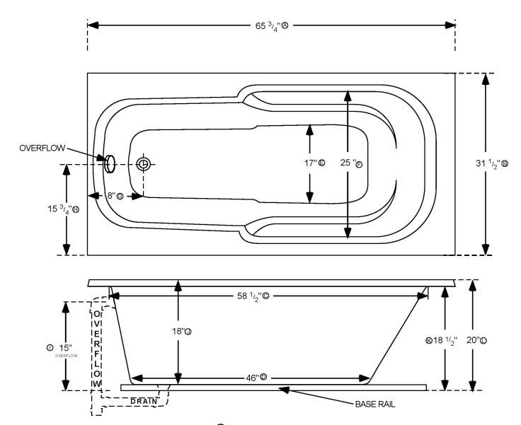
INSTALLATION: Add 1/2" to 1" height of tub at point (b) to allow space for bedding compound. All Watertech Whirlpool Baths require mortar to be placed under tub for tub bedding. Please measure tub before building tub cabinet. Drawing shows standard pump location for this tub. Custom pump locations available - please call Watertech Whirlpool Baths for details. Measurements are plus or minus 1/2", and are subject to change without notice.
