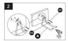
Re-screw toggle end to toggle bolt (CC) and insert both toggle ends into drilled holes. Tighten toggle bolts (CC) to secure to wall.
