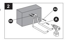
3. Using screws (AA), secure the hanger (A) to the wall by screwing into the anchors (BB).
