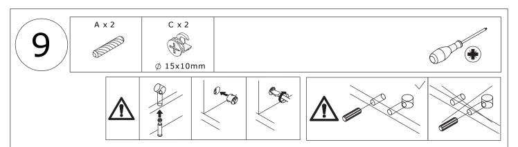
Connect board 7 and 9 with board 14 using wooden dowel(A) and turn cam lock(C) clockwise to tighten as shown.
