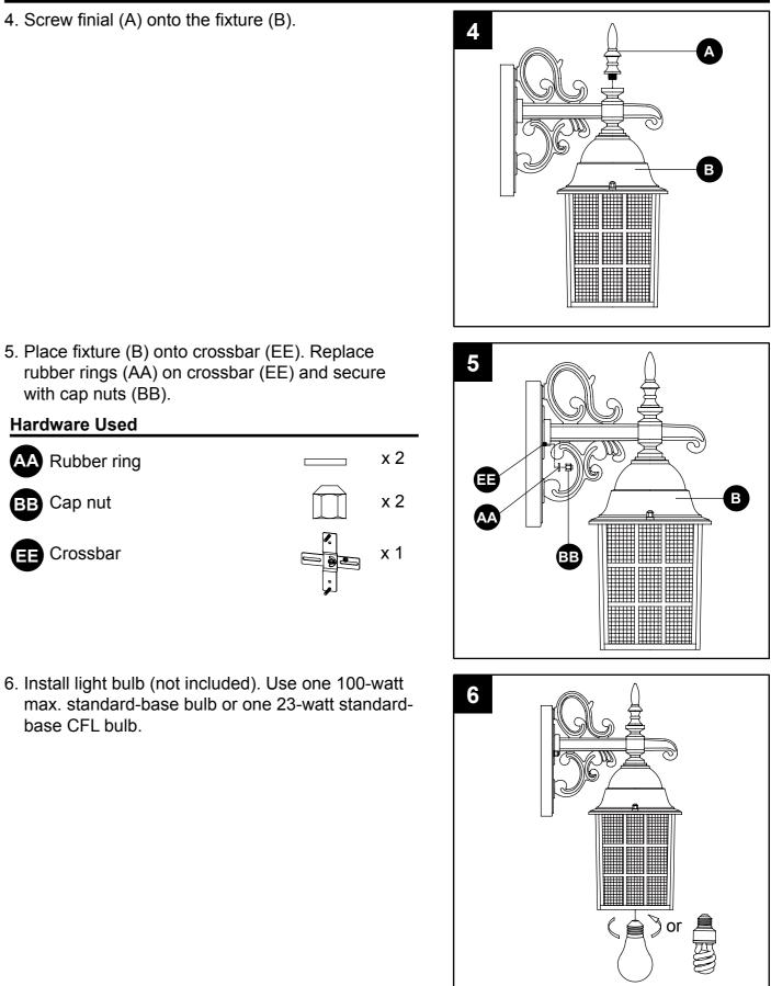
• Note: Before use, add silicone glass sealant between wall and canopy, leaving the bottom clear so moisture can drip down.
