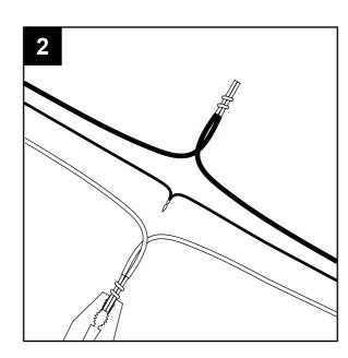
3. Attach wire nuts (CC). Tape wire nuts (CC) and wires together.
