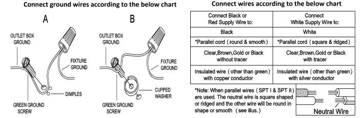
Twist the wires together with plastic wire connector (A) until tightly joined, then carefully tuck all wires into the outlet box
